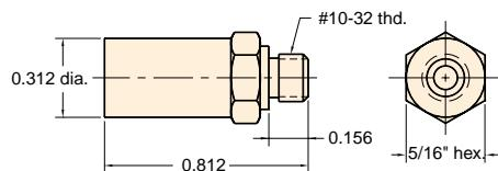
**Material:** Nickel plated brass body sintered stainless steel muffler (60 micron)
